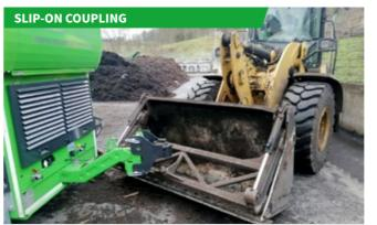
The sturdy slip-on coupling for the drawbar permits safe movement of the trommel screen with construction site vehicles.
