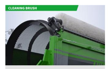
The hydraulically folding cleaning brush travels along above the screening drum, thus preventing the damaging build-up of residues.
