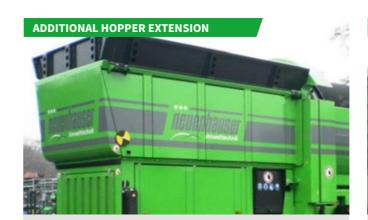
The extension of the feed hopper increases the capacity for screening wood chips, bark, domestic waste, coal, industrial waste and other materials.
