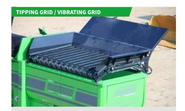
By screening out coarse impurities from construction debris, top soil or other materials, this option effectively prevents possible damage to the drum.
