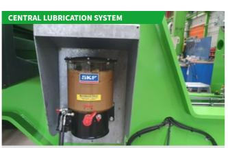
The automatic central lubrication system ensures the reliable operational readiness of the trommel screen by constant renewal of the lubricating film.
