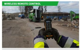
To significantly reduce the time and personnel required, the remote control allows comfortable control of the star screen even from the wheel loader.
