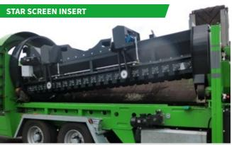
The screening drum can be easily exchanged for the star screen insert in order to utilize the strengths of star screen technology for specific tasks.
