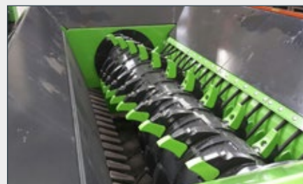
Adjustable cutting gap for consistent result
