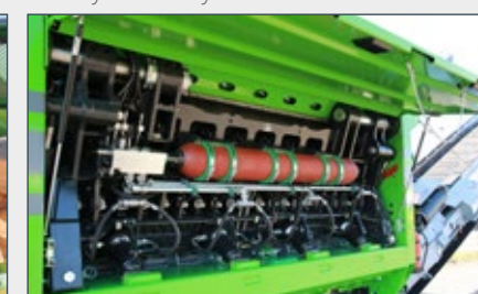
Hydraulically secured counter comb
